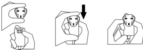
Connect the USB cable to the A/C adapter that came with the Tractive® GPS device. Then attach the charging clamp on the device as shown in the image below.
